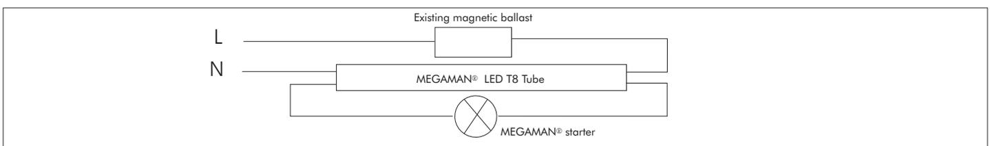
If magnetic ballast and starter are not available, an alternative wiring method is shown below:
