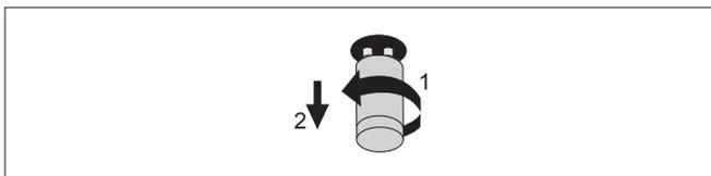
Step 6: Install MEGAMAN® LED T8 Tube into the lamp holder
