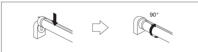
Step 2 & 3: Remove the conventional lamp by turning 90°
